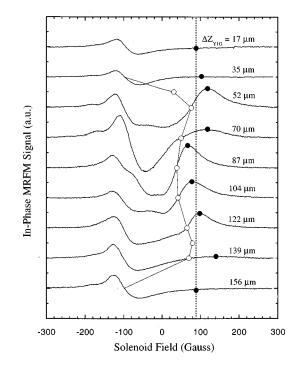
FIG. 2. Series of FMR spectra as a function of solenoid field are shown for several values of  $\Delta z_{\text{YIG}}$ : the positions of the maximum deviation ( $\bullet$ ) and the center of the additional signal ( $\bigcirc$ ) are shown. The dotted line indicates the value of the solenoid field at which the signal intensity as a function of  $\Delta z_{\text{YIG}}$  (shown as a dotted line in Fig. 3) is determined.
