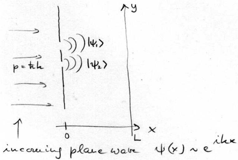
At  $x=0$ , the plane wave gets blocked by the screen, except for the holes. Let's call the state corresponding to the wave generated behind the screen from electrons passing through the upper slit as  $|\psi_1\rangle$ , and similarly  $|\psi_2\rangle$  for the state corresponding to electrons passing through the lower slit.
