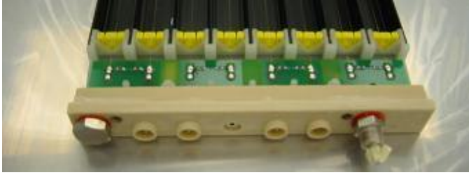
(b) Endcap with HV and gas connectors.
