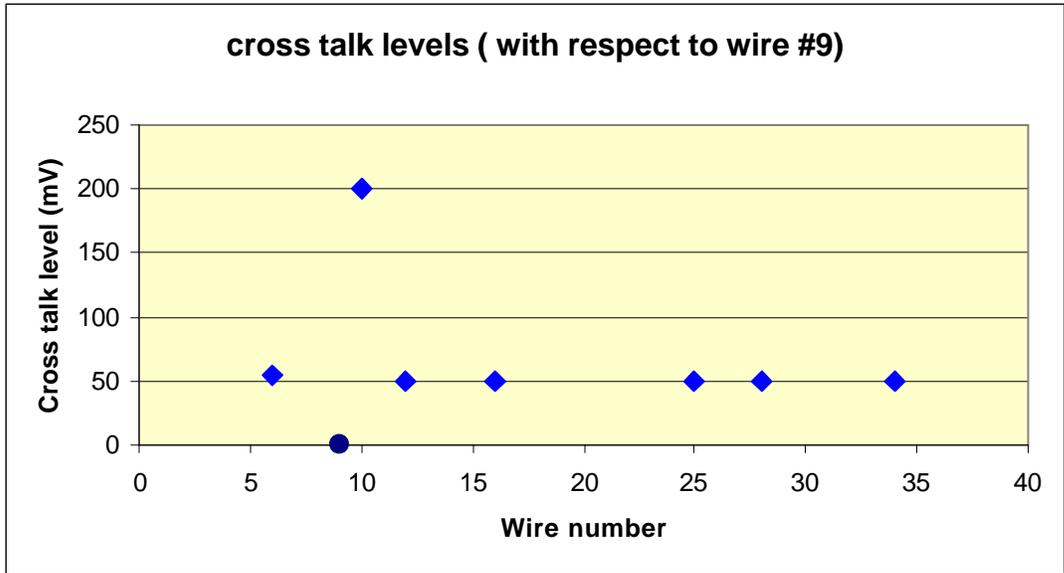
Except for wire #10, ie the neighboring wire the cross talk is very small. This test measures the wire to wire cross talk. We are more interested in the wire to wire to strip cross talk. To study this effect we brought our setup to the LST tubes. With one wire of the Kerpen cable connected to the pulse generator and another wire connected to a HV pin in the tube endcap we record the signals on the strip above the corresponding wire.
