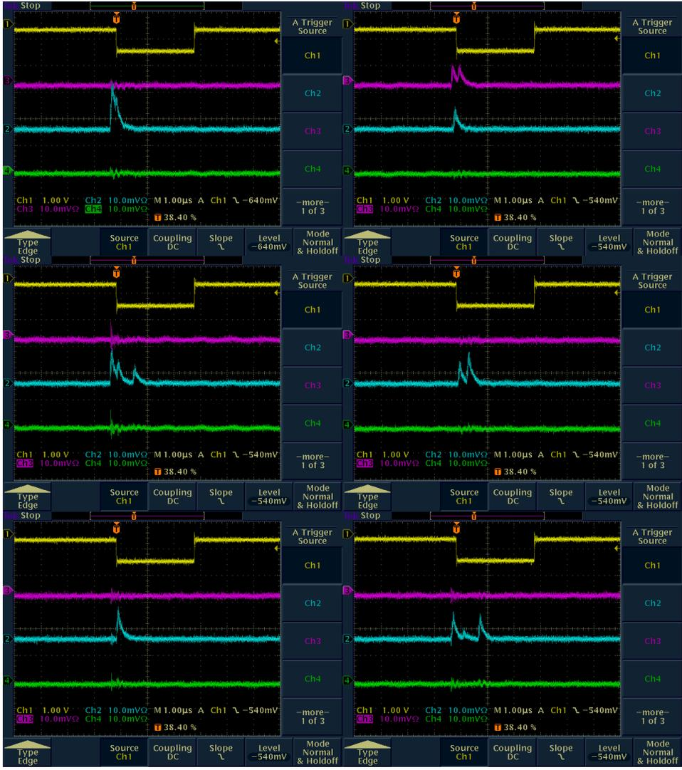
Same configuration as before but this time without the 82 Ohm termination resistor.
