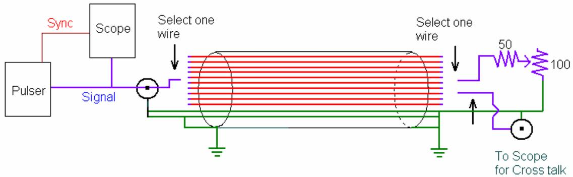
The Kerpen cable is not a coax cable and hence does not provide constant impedance. The impedance of a particular wire depends its location with respect to the ground shield and the ground wires in the cable bundle. We picked a random combination and checked some ten wires to obtain the following results:
