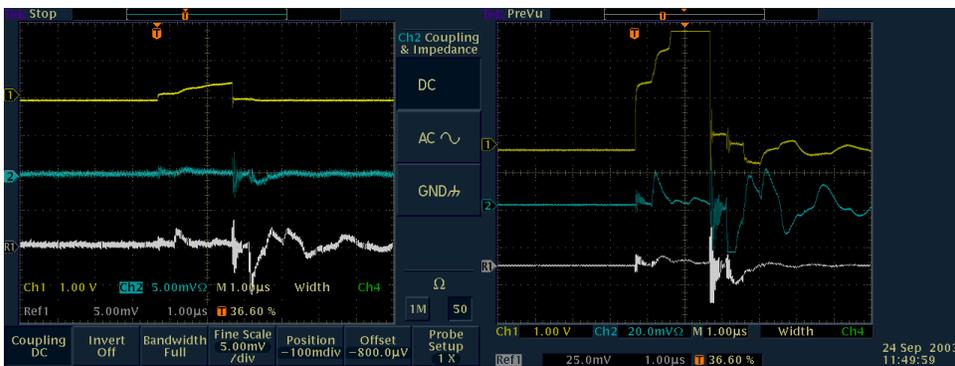
The observed cross talk is very small. It can be further reduced by terminating the HV cable at the power supply end with 80 – 100 Ohm which matches the average impedance.
