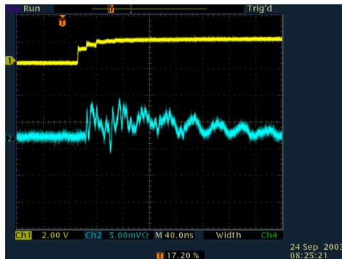
Same configuration but wire #6 and #16 are now connected at the far end (which would be the case if the two wires share the same HV channel).
