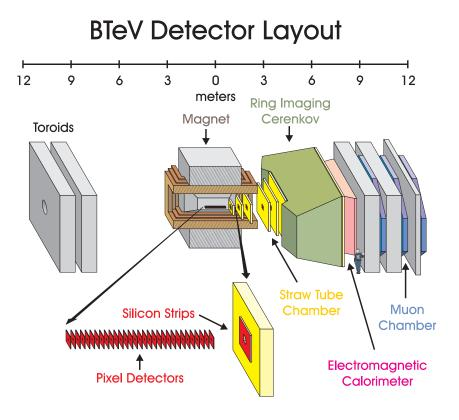
Figure 1: Schematic view of the BTeV Spectrometer.
