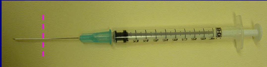
Needle 25G (ID = 0.254 mm, OD = 0.5mm, SS\_steel wall = 0.127 mm)
