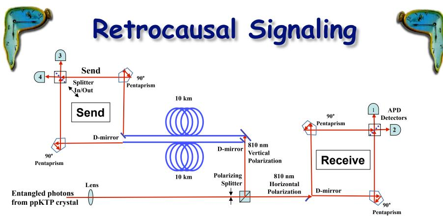
We have 10 km of high quality optical fiber coiled in the corner of the laboratory. We split the V-polarized entangled photon beam with a D-mirror, and pass each of the two paths of entangled photons through 10 km of fiber.
