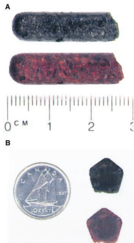
Fig. 3. (A) Photographs of the bulk organometallic polymer before (bottom) and after (top) pyrolysis at 600°C. (B) Photographs of the CPPN cast in a pentagonal Teflon mold before (bottom) and after (top) pyrolysis at 600°C. The ceramics retain the shape of the precursor polymer and show only a small contraction after pyrolysis (pyrolysis was not performed in a mold).
