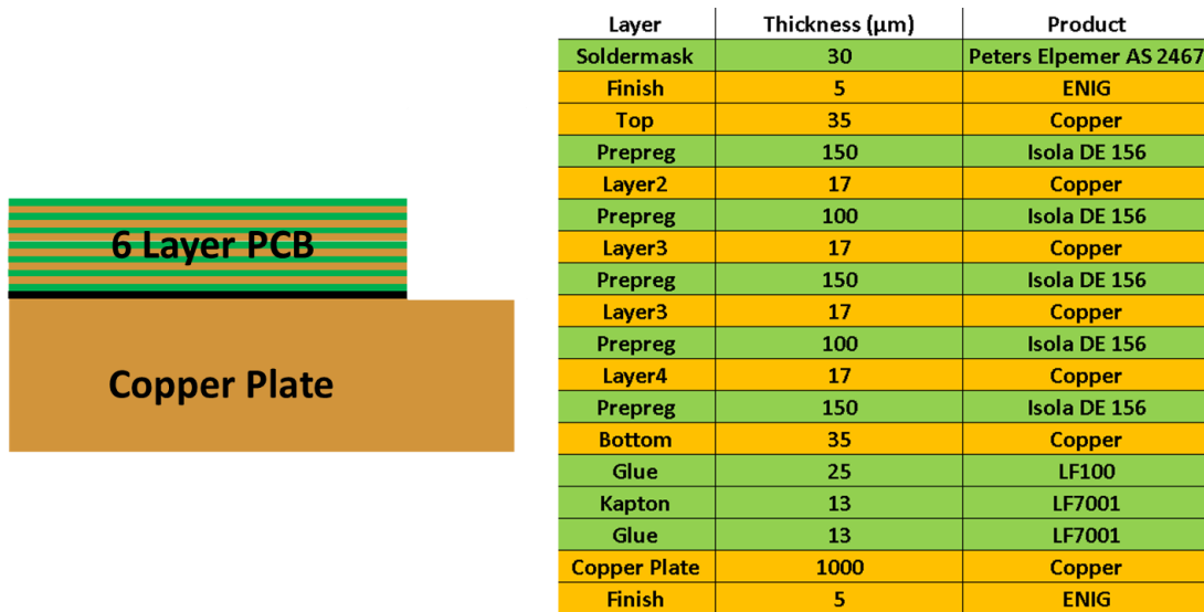
Figure 2: Simplified cross section of the opto-board (left). Complete listing of opto-board stack up information (right).
