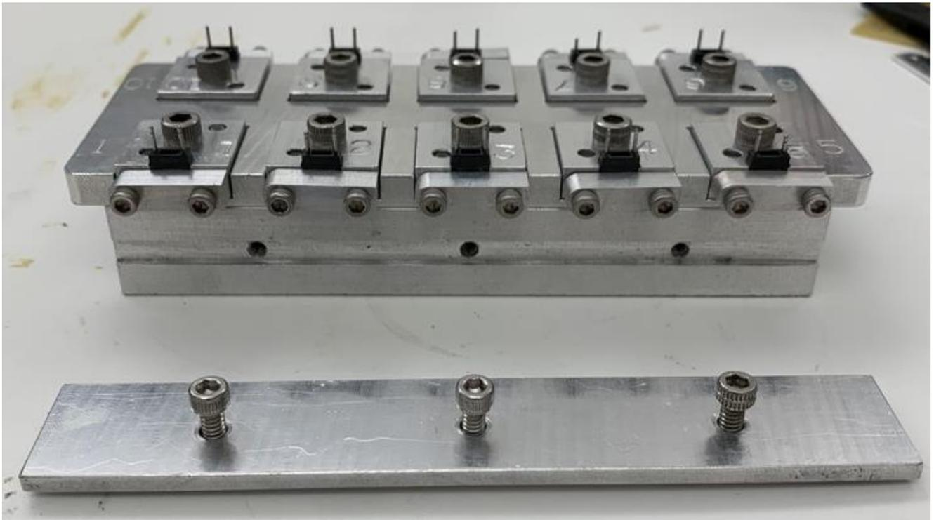
Figure 5: The opto-pack base alignment jig with sidebar.
