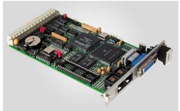
Embedded VME Computer: Prototype system achieved 3 Mbit/s loading Spartan FPGA
