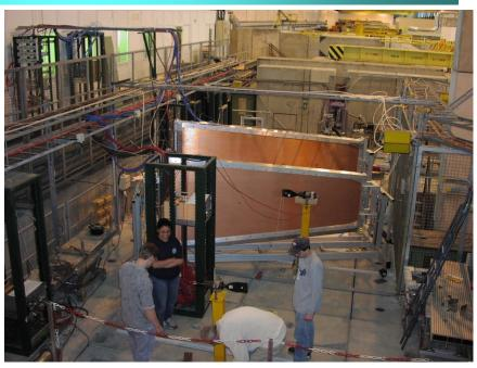
DAQ rate tests carried out with high intensity pion beam.
