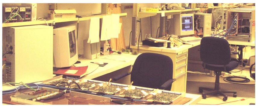
PC boards will be etched and stuffed commercially Boards will be measured and debugged on computerized tester before and after burn-in at OSU
