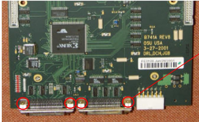
These screws were put on after the board was tested by a technician. Apparently they were not tight enough.
