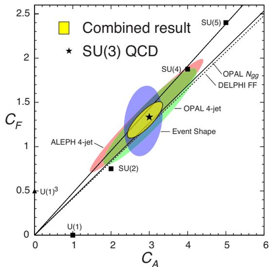
Fig. 7. Determinations of the color factors  $C_F$  and  $C_A$  from studies of event shapes, jet cross sections, and fragmentation functions at LEP (adapted from Ref. 324). The common fit, shown as the shaded ellipse, favors the QCD expectations indicated by  $\star$ , and discriminates against other hypotheses. The error ellipses show the 90% confidence level.
