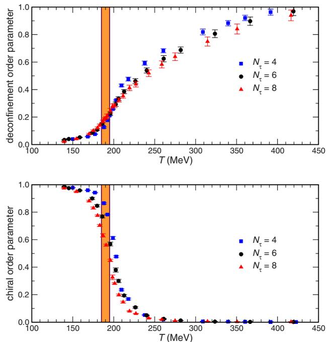
Fig. 11. Order parameters for deconfinement (top) and chiral symmetry restoration (bottom) as a function of temperature. The physical temperature  $T = a/N_\tau$ , where  $a$  is the lattice spacing. Agreement for several values of  $N_\tau$  thus indicates that discretization effects from the lattice are under control. From Refs. 477 and 478.
