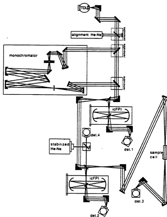
Figure 3: Optical schematic of the tunable diode laser spectrometer system used in these experiments. The cell shown in Fig. 2 replaces the sample cell in this figure.
