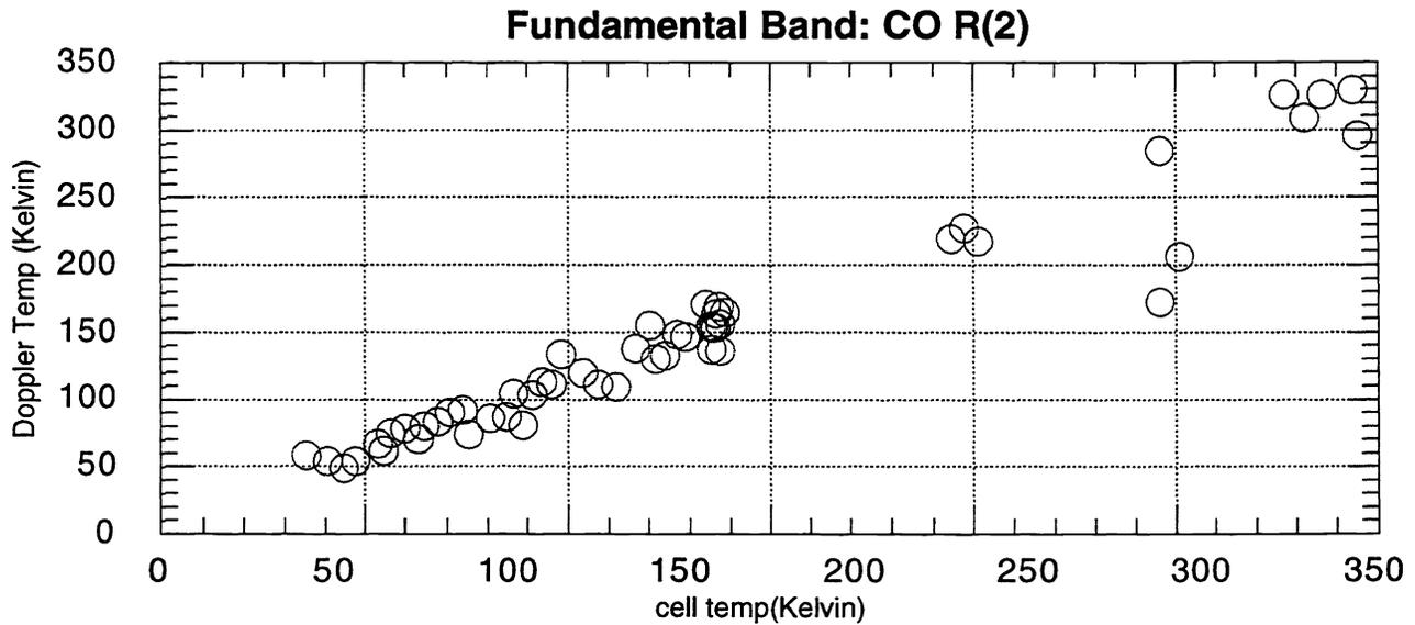
Figure 5: A plot of gas temperature calculated from the Doppler width for the R(2) line of CO versus cell temperature
