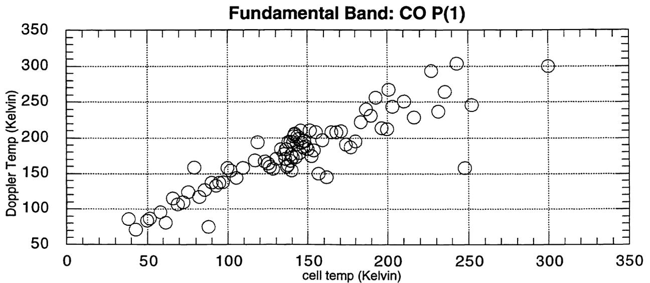
Figure 6: A plot of gas temperature calculated from the Doppler width for the P(1) line of CO versus cell temperature
