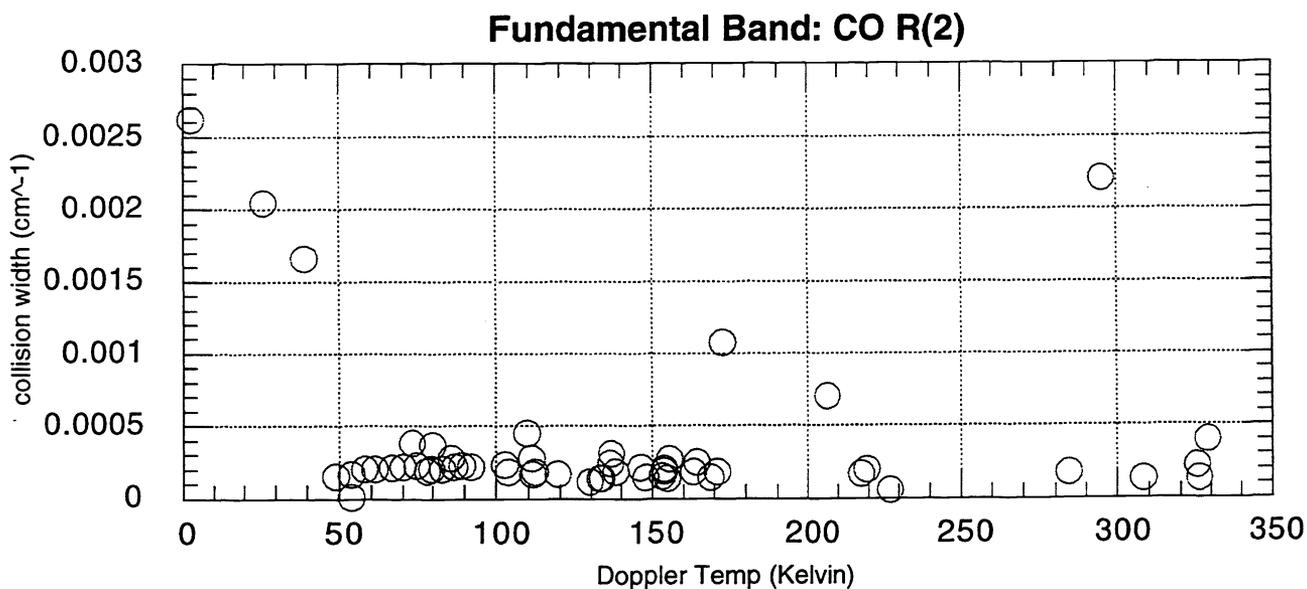
Figure 7: A plot of the Lorentzian, or collision, width for the R(2) line of CO versus Doppler temperature
