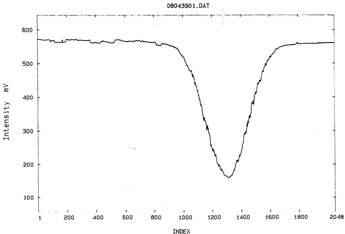
Figure 4: A typical low temperature spectrum of CO recorded using the low temperature cell described in this paper. The spectrum shows absorption by the P(5) line in the CO fundamental band. Cell temperature was 37 Kelvin, and gas pressure was 139 milliTorr.
