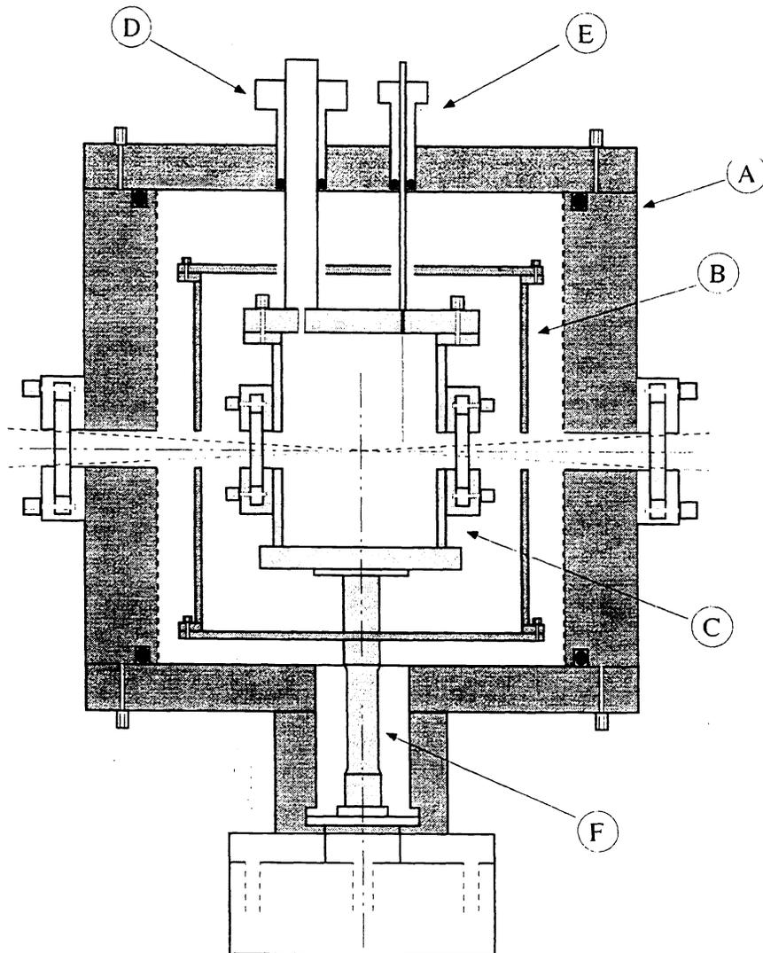
Figure 2: Schematic diagram, in cross section, of the low-temperature cell used for these experiments and described in detail in the text.
