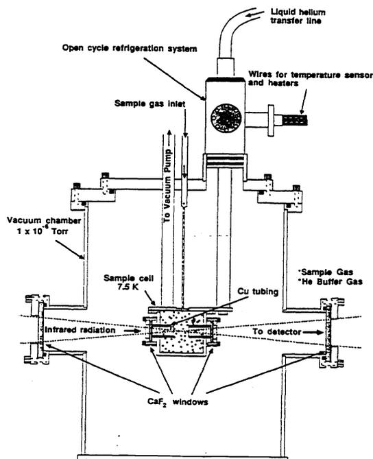
Figure 1: Schematic diagram, in cross section, of the low-temperature absorption cell as it was configured for the experiment described in reference 15. Calcium Fluoride windows replaced the usual microwave windows, and microwave waveguides were removed.
