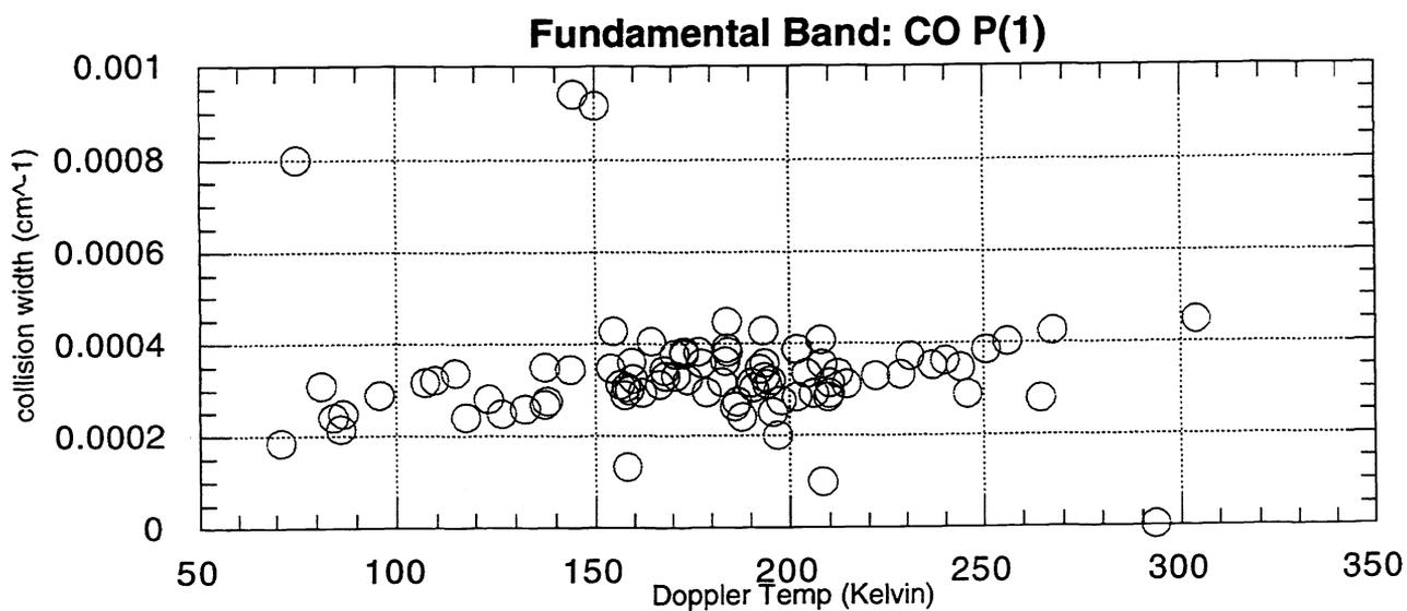
Figure 8: A plot of the Lorentzian, or collision, width for the P(1) line of CO versus Doppler temperature
