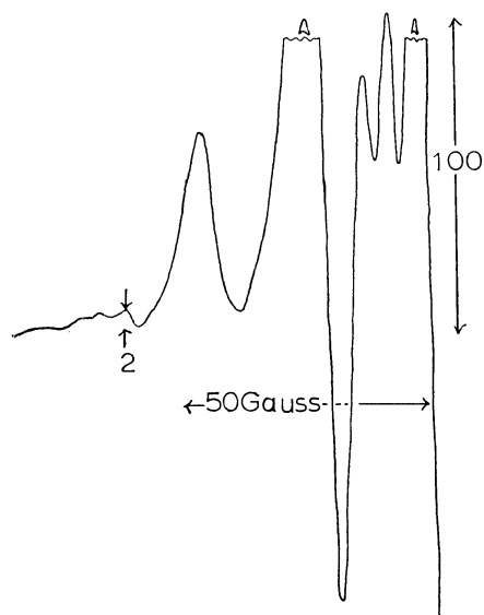
Fig. 3. Carbon-13 lines of the spectrum obtained from an irradiated single crystal of methacrylamide. \angle xH = 90^\circ , \angle yH = 30^\circ . Only the left half of the spectrum is shown. The ^{13}\text{C} splitting constant has been reported as 35 gauss. 4
