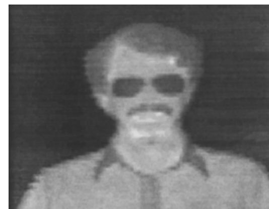
Indoor Passive Image at 700 GHz (0.3 K bolometer)
