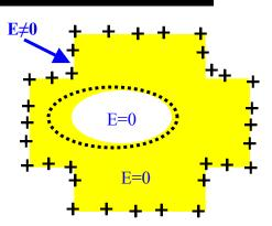
Conductor with net positive charge. Cross-section-view.
