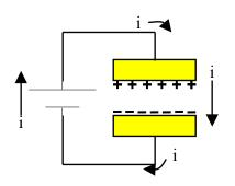
• An initially uncharged capacitor effectively acts likes a wire when it first starts to charge because pulling the first electron off is easy.
