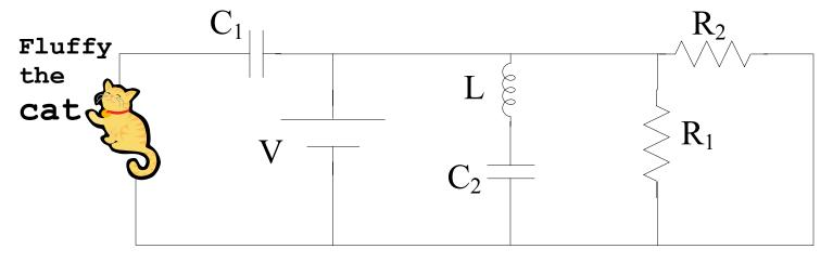
Inductor L and capacitor  $C_2$  are in series. (Don't know what an inductor is yet? Doesn't matter. It's still in series with  $C_2$ !)
