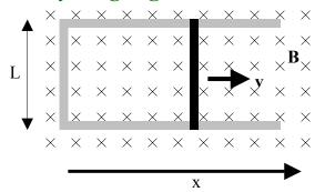
The rail has mass M and resistance R and is moving at constant speed v.
