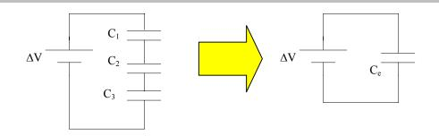
$$\Delta V = \Delta V_1 + \Delta V_2 + \Delta V_3 \quad {\rm True \ for \ any \ set \ of \ components \ in \ series \ !!!}$$
