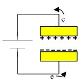
When charging or discharging we will treat capacitors as having a current even though, in reality, no electrons ever jump the gap from one plate to the other.
