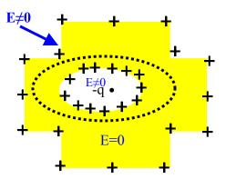
Conductor with net positive charge and a cavity charge.
