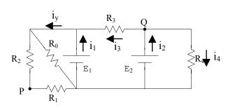
$E_1 = 10V$ ,  $E_2 = 20V$   $R_0 = R_1 = R_2 = 100 \Omega$ .  $R_3 = 300 \Omega$ ,  $R_4 = 400 \Omega$ .
