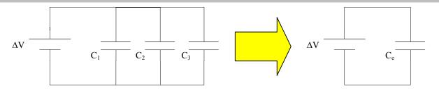
$$\Delta V = \Delta V_1 = \Delta V_2 = \Delta V_3$$
