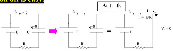
• A fully charged capacitor blocks steady state currents. It acts like a broken wire.
