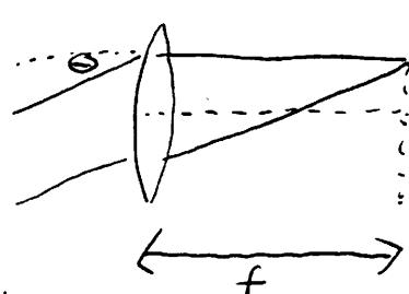
$$\left( \begin{array}{c} n \\ r \end{array} \right) = \left( \begin{array}{cc} 1 & 0 \\ 0 & 1 \end{array} \right) \left( \begin{array}{c} n \\ r \\ z \\ z-f \end{array} \right) \quad \left. \right\} \quad I(r) \rightarrow I(\theta)$$
