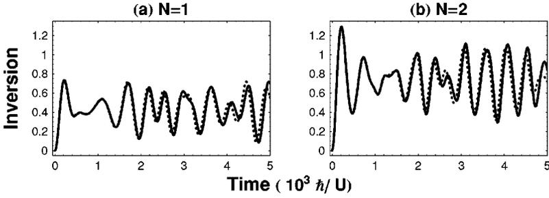
FIG. 6. Time-dependent inversion  $\mathcal{S}(t)$  for (a)  $N=1$  and (b)  $N=2$  junctions given that the initial state of the resonator is a coherent state with  $\langle n \rangle = 2$  and the junctions are initially in their ground states. The solid line denotes the full numerical solution, and the dotted line follows from the two-level approximation.
