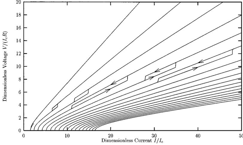
FIG. 2. Current-voltage ( $IV$ ) characteristics for arrays of sizes  $N=2$  to 19 (increasing from left to right) with the inverse inductance parameter  $\lambda=100$ . In the hysteretic regions, arrows indicate that the voltage is measured as the current is being increased from zero, or decreased from a high value.
