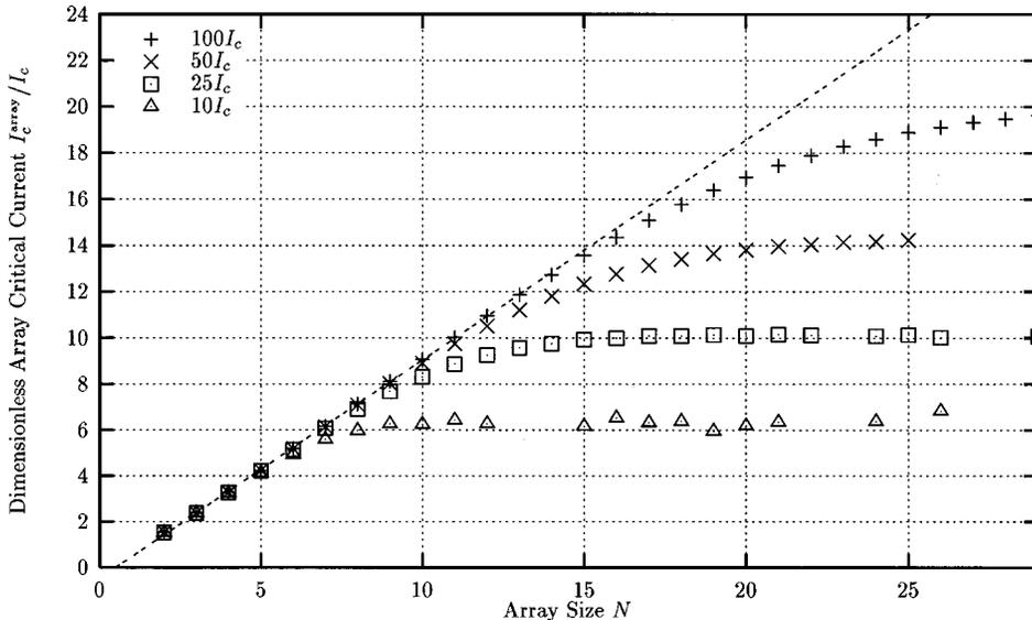
FIG. 3. Critical current  $I_c^{\text{array}}$  as a function of number of wires  $N$  in each layer, plotted for several  $\lambda=100, 50, 25,$  and  $10$  as indicated. The straight line has slope  $I_c$ , the critical current of a single vertical junction.
