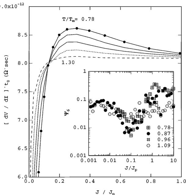
FIG. 3. Simulated  $dV/dI$  for  $T/T_m = 0.78, 0.87, 0.96, 1.087,$  and  $1.30$  near melting. Inset shows  $\Psi_6$ . The crossing of all the  $dV/dI$  curves near  $J/J_p \sim 0.12$  coincides with the dip in  $\Psi_6$ .
