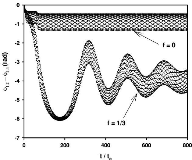
FIG. 4. Difference between the Josephson phase drops across two junctions on the top row of a  $3 \times 3$  array as a function of dimensionless time.  $I_B/I_c=2.0$ ,  $\beta_c=0$ . Both  $f=1/3$  and  $f=0$  are shown. An identical perturbation is applied to the phase at each superconducting node at  $t/t_c=60$ . This *overdamped* array is neutrally stable for both values of  $f$ .
