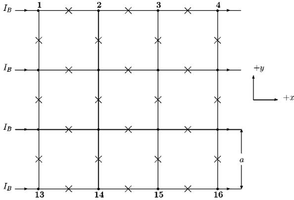
FIG. 1. Schematic of a square array with  $3 \times 3$  plaquettes. An  $N \times N$  array has  $(N+1) \times (N+1)$  nodes, some of which are numbered in the figure. The dc bias current is applied and removed horizontally ( $x$  direction) and a constant magnetic field is applied in the  $+z$  direction. Each junction has a resistance  $R$ , a capacitance  $C$ , and a critical current  $I_{c,jk}$ , where  $j$  and  $k$  index the nodes on either side of the junction.
