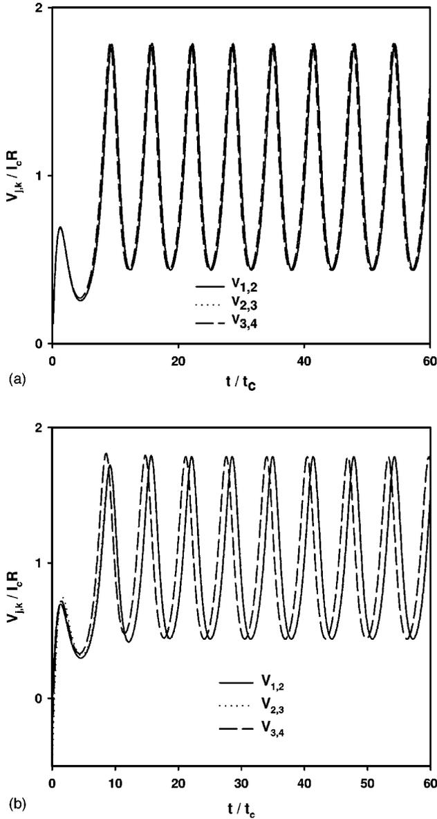
FIG. 2. Dimensionless voltage across each of the three junctions in the top row of a  $3 \times 3$  array, plotted versus dimensionless time. (a)  $I_B/I_c = 1.2$ ,  $\beta_c = 1.0$ ,  $f = 0$ . All voltages were initialized to zero. (b)  $I_B/I_c = 1.2$ ,  $\beta_c = 1.0$ ,  $f = 0$ . All voltages were initialized randomly between zero and 1.
