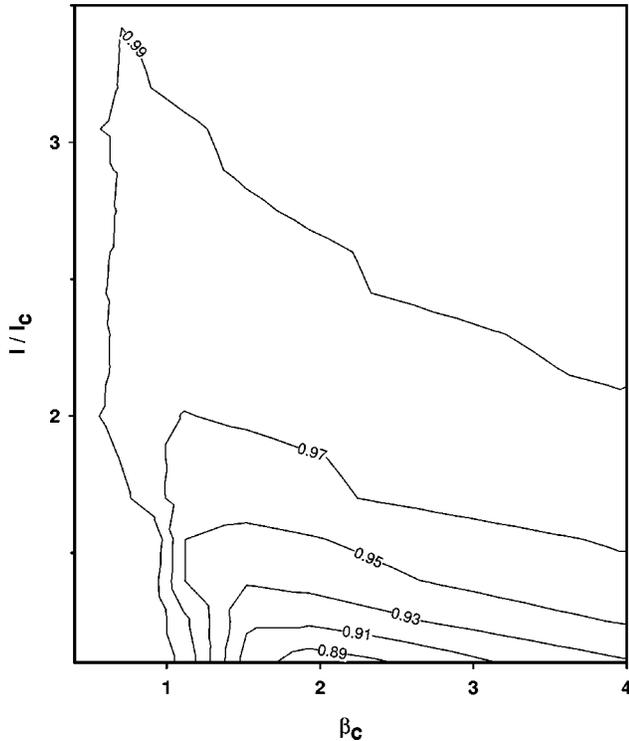
FIG. 6. Contour plot of largest Floquet multiplier as a function of bias current and junction capacitance for a  $5 \times 5$  array, at  $f = 1/3$  with no disorder. The  $\mu = 0.99$  contour may be thought of as the boundary between stable ( $\mu < 0.99$ ) and unstable ( $\mu > 0.99$ ) synchronization. Note the similarity between the contour lines in this figure and those of Fig. 5.
