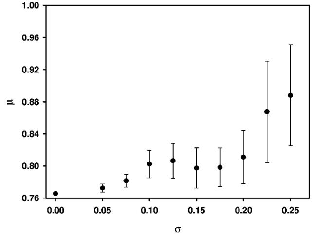
FIG. 7. Largest Floquet multiplier as a function of standard deviation of critical currents in a disordered  $3 \times 3$  array, with  $I_B/I_c = 1.25$ ,  $\beta_c = 1.0$ ,  $f = 1/3$ . These parameters resulted in stable phase locking in the uniform array [cf. Fig. 5].
