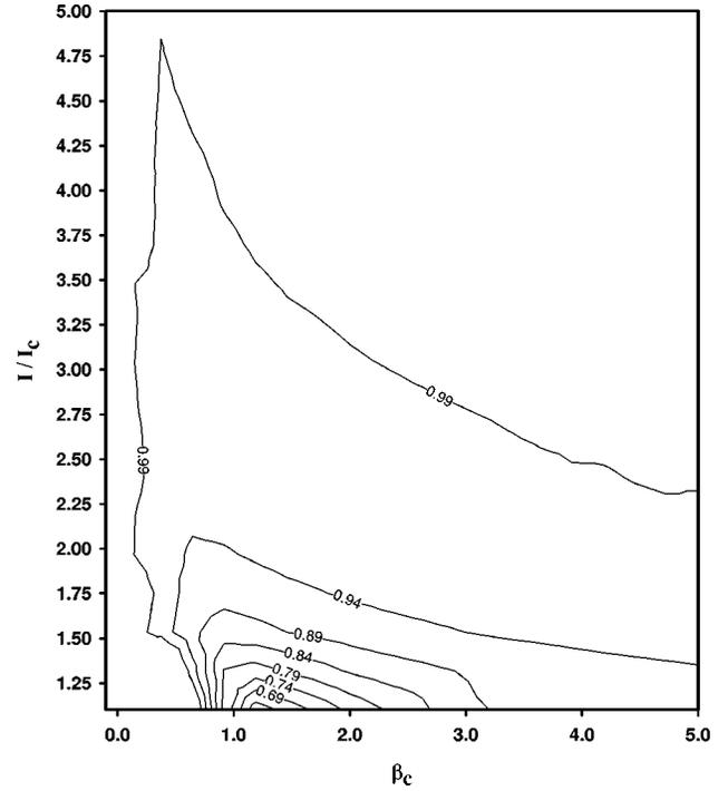
FIG. 5. Contour plot of largest Floquet multiplier as a function of bias current and junction capacitance for a  $3 \times 3$  array, at  $f=1/3$  with no disorder. The  $\mu=0.99$  contour may be thought of as representing the boundary between stable ( $\mu < 0.99$ ) and unstable ( $\mu > 0.99$ ) synchronization.
