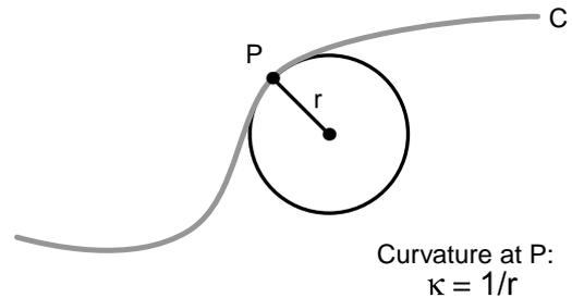
Fig. 11. Radius of curvature. The most common method of measuring the magnitude of curvature at any point ( $P$ ) on a curve is to specify the radius ( $r$ ) of the circle that most closely conforms to the shape of the curve at that point. This is also referred to as the osculating circle.
