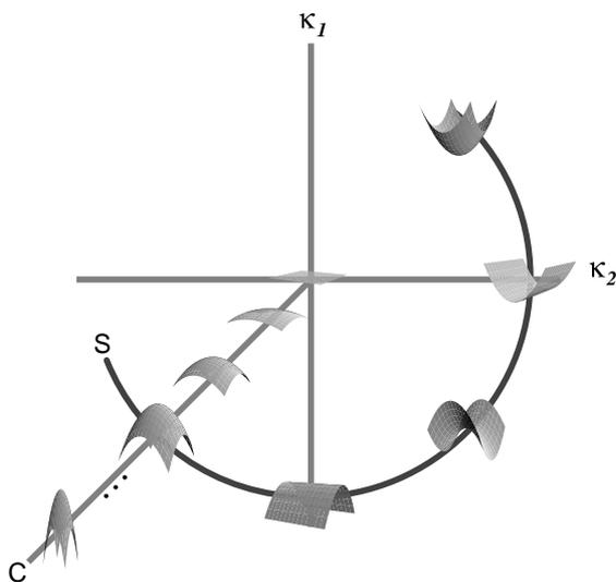
Fig. 3. The effects on surface structure from variations in the curvedness ( $C$ ) and shape index ( $S$ ) parameters of curvature, and the relation of these components to the principal curvatures ( $\kappa_1$  and  $\kappa_2$ )—adopted from Phillips and Todd (1996).
