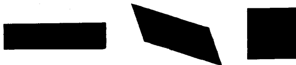
Figure 3. The optical projection of an elongated rectangular surface element at a 60° slant. (From left to right the depicted tilts relative to the horizontal are 0°, 45°, and 90°, respectively.)
