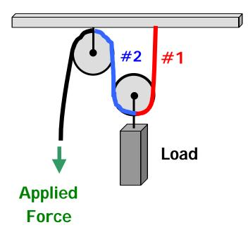
This pulley system has two attached ropes, so its theoretical mechanical advantage = 2
