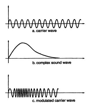
Because FM radio works on the principle of frequency modulation, the actual frequency of the transmission will vary. Therefore, instead of broadcasting at a single frequency, FM radio broadcasts over a range of frequencies. The range of frequencies over this bandwidth is small compared to the frequency of the FM carrier wave. This means that the FM station can still be assigned a single frequency.
