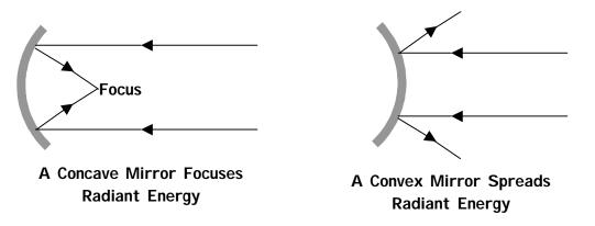
Figure 3.1 Radiant Energy Reflecting from Mirrors
