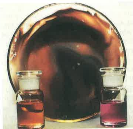
▲ Figure 11.44 Solutions of fullerenes. Unlike diamond and graphite, the new molecular forms of carbon can be dissolved in organic solvents. The orange solution on the left is a solution of C_{70} in n -hexane, which is a colorless liquid. The magenta solution on the right is a solution of buckyball, C_{60} , in n -hexane.
